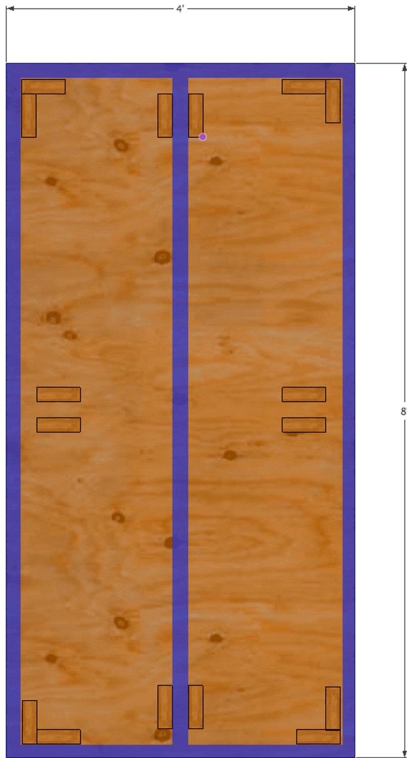
Diagram shows how jig is used to create a wall panel with vertical support beam. This shows how the scrap wood is used to guide the wood into place.
