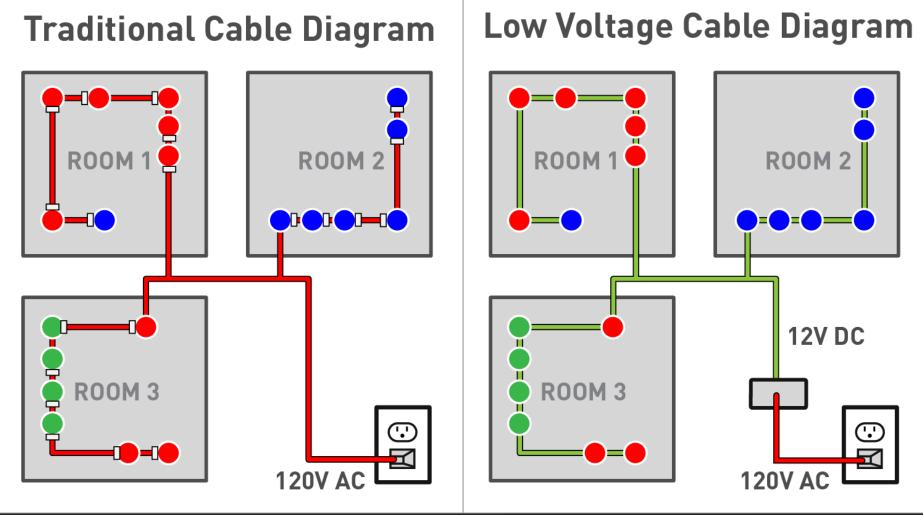
20 LEDs @ 20mA/LED= 400mA = 0.4A 12V Power Supply > 0.4A current output OK **Topic :** LED Systems
